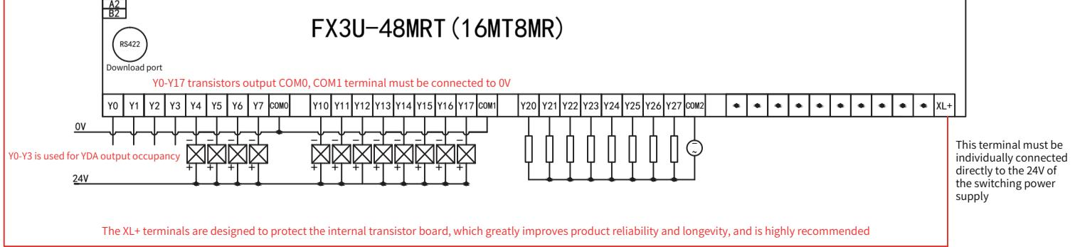
The XL+ terminals are designed to protect the internal transistor board, which greatly improves product reliability and longevity, and is highly recommended.
