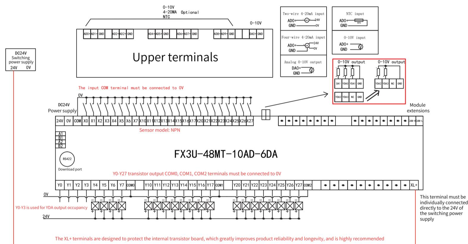
The XL+ terminals are designed to protect the internal transistor board, which greatly improves product reliability and longevity, and is highly recommended.
