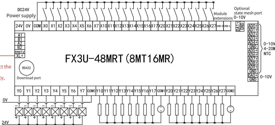
The XL+ terminals are designed to protect the internal transistor board, which greatly improves product reliability and longevity, and is highly recommended
