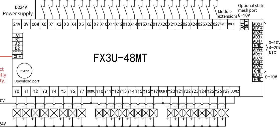
This terminal must be individually connected directly to the 24V of the switching power supply
